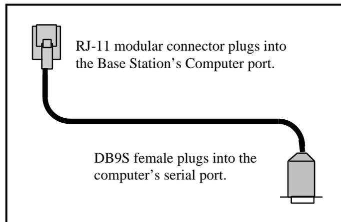
Figure D-3 9-Pin Serial Port Cable
