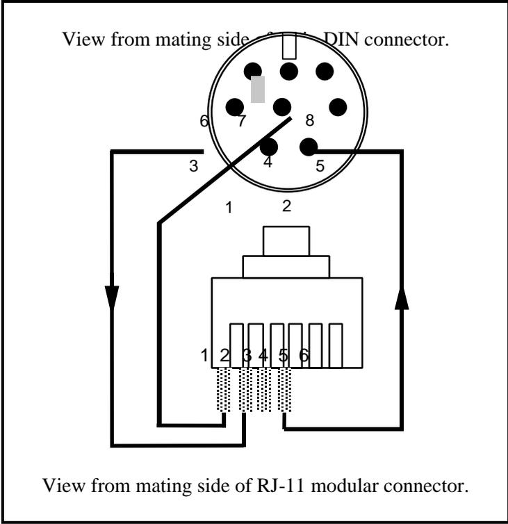
Figure D-6 DIN 8 Serial Port Cable Pin Configuration
