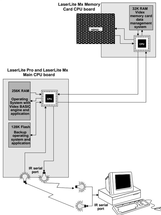
Figure 1-4 LaserLite Pro and LaserLite Mx System Components
