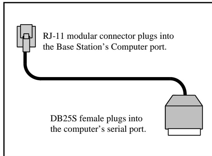
Figure D-1 25-Pin Serial Port Cable
