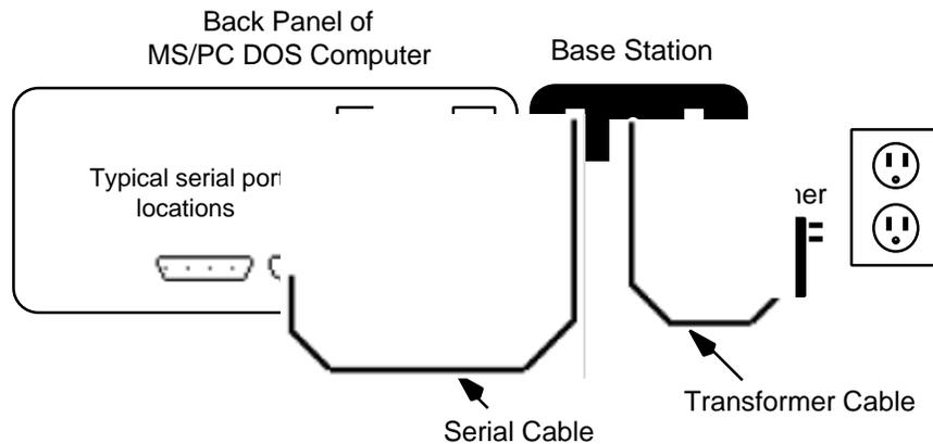
Figure 1-12 Base Station Connections
