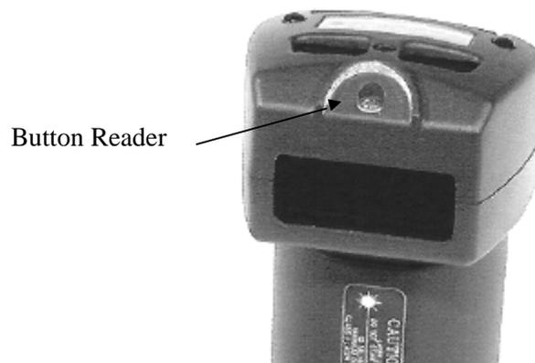
Figure 1-8 LaserLite Pro/LaserLite Mx Button Reader
