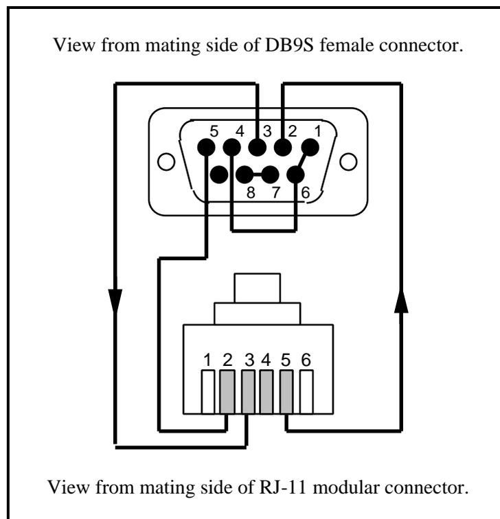
Figure D-4 9-Pin Serial Port Cable Configuration
