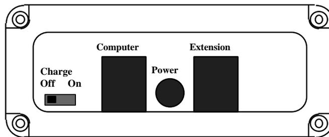
Figure 1-11 LaserLite Pro/Mx Base Station - Side View
