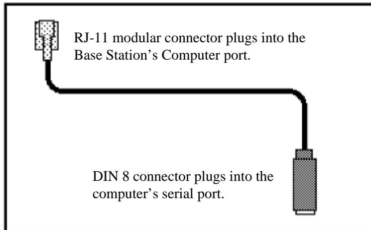
Figure D-5 DIN 8 Serial Port Cable
