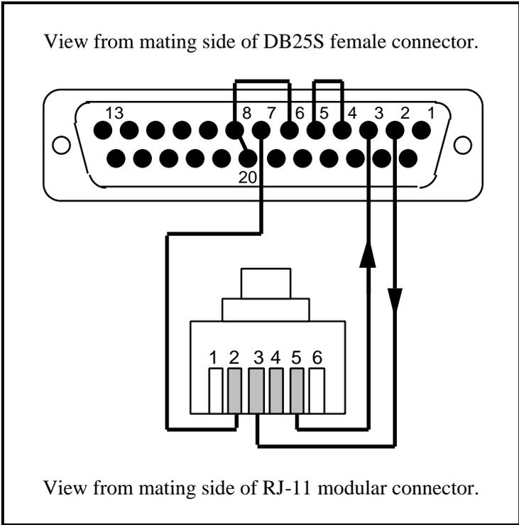
Figure D-2 25-Pin Serial Port Cable Configuration
