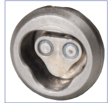
Figure 1 – Dirty Lock Face
